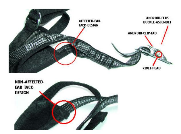
Androids shipped during this time may be prone to the Android Clip Tab moving past the rivet. The clip tab may move past the rivet head and prevent the Android Clip from properly closing and opening. If you have an Android that meets this critera, please contact your local Black Diamond Dealer, the location where you purchased the Android, or the Black Diamond Warranty department for a replacement component. Replace the Android Clip Assembly and thread the webbing as shown.
